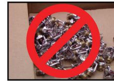
INCORRECT (Stored loose in a box)
