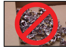
INCORRECT (Stored loose in a box)
