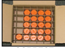
CORRECT (Protective caps in place)
