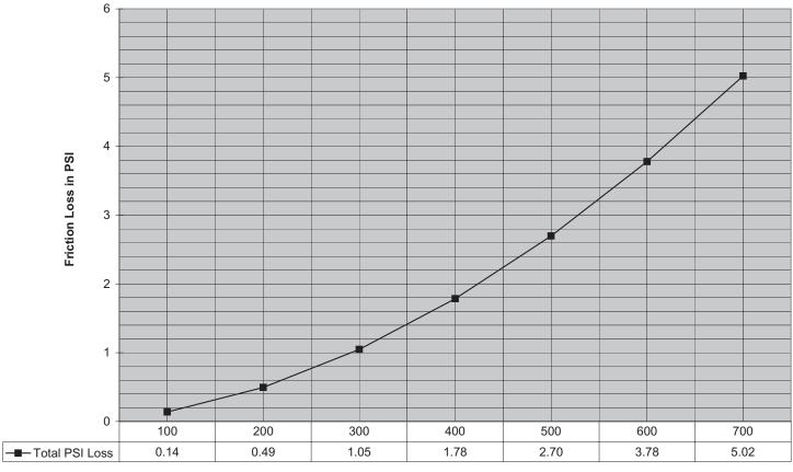
Flow in GPM (C = 120)
