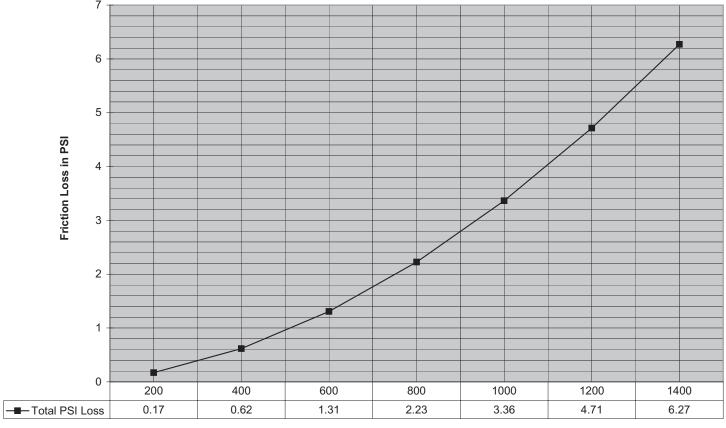
Flow in GPM (C = 120)
