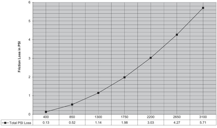
Flow in GPM (C = 120)
