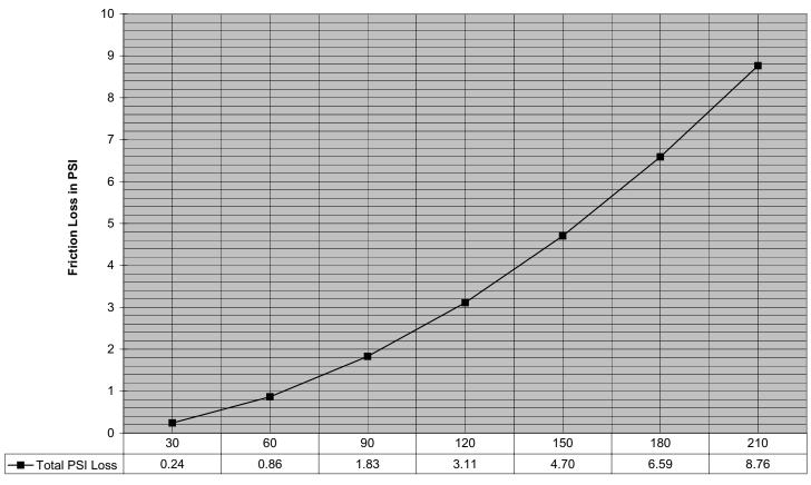
Flow in GPM (C = 120)
