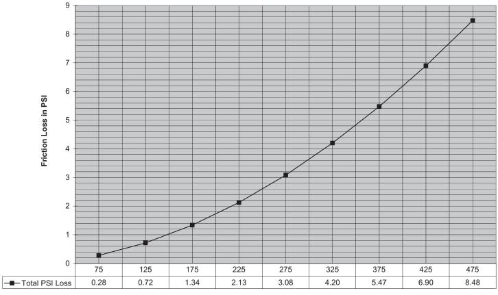
Flow in GPM (C = 120)
