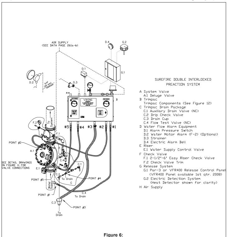
Surefire® Double Interlock Preaction System 2-1/2" - 6" Straight Through Vertical Valve
