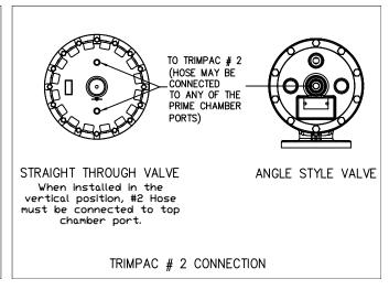
**Figure 11: Valve Connections**
