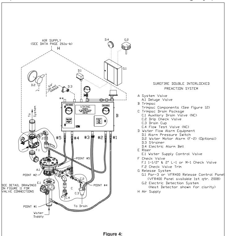
Surefire® Double Interlock Preaction System 2", 3", 4" & 6" Angle Style Valve
