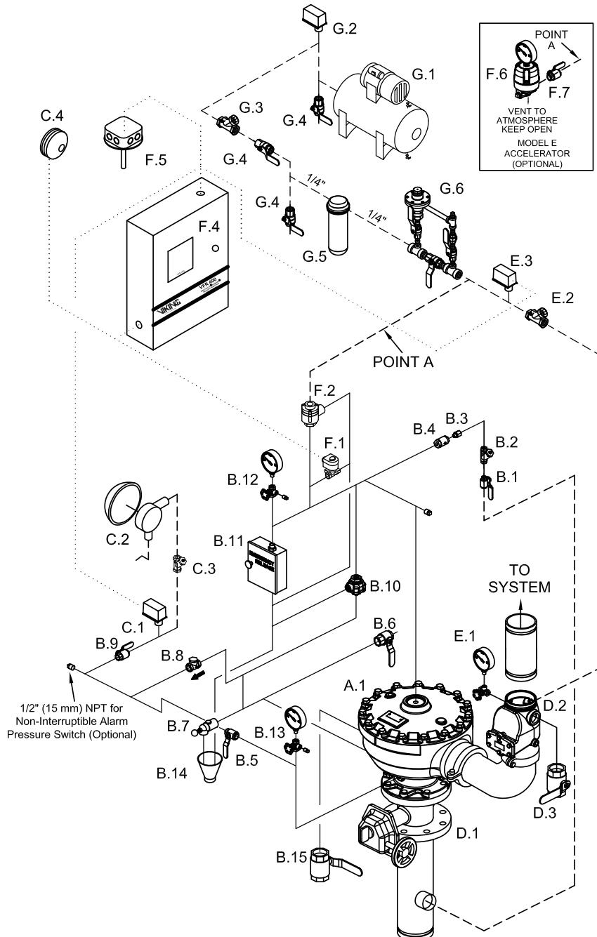
— — — Dashed lines indicate pipe required but not listed in "System Components" Table.
