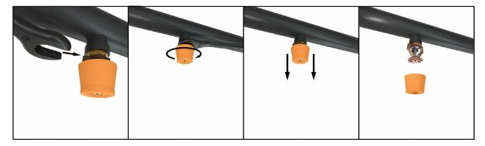
Figure 5: Sprinkler Installation
