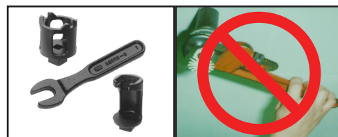
CORRECT (Special installation wrenches)
