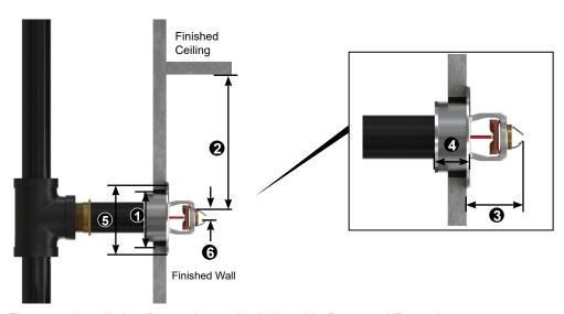
Figure 4: Installation Dimensions with Adjustable Recessed Escutcheon
