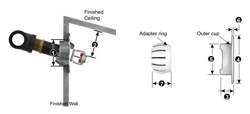
Figure 5: Installation Dimensions with G-1 Escutcheon
