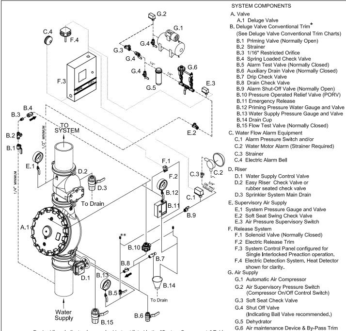
Dashed lines indicate pipe required but not listed in the "System Components" Table.
