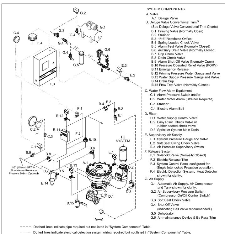
FIGURE 1: ANGLE DELUGE VALVE WITH TANK-MOUNTED COMPRESSOR
