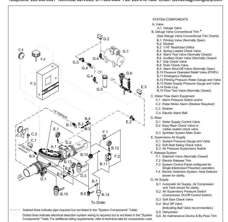
FIGURE 5: HORIZONTAL DELUGE VALVE WITH TANK-MOUNTED COMPRESSOR
