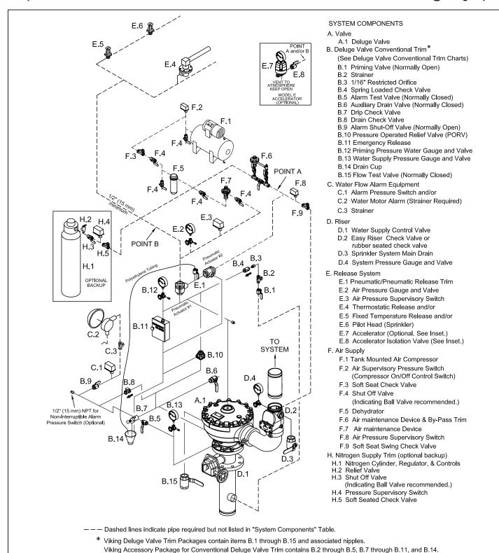
FIGURE 1: Angle Style Valve with Tank-Mounted Compressor (6" Valve Shown)
