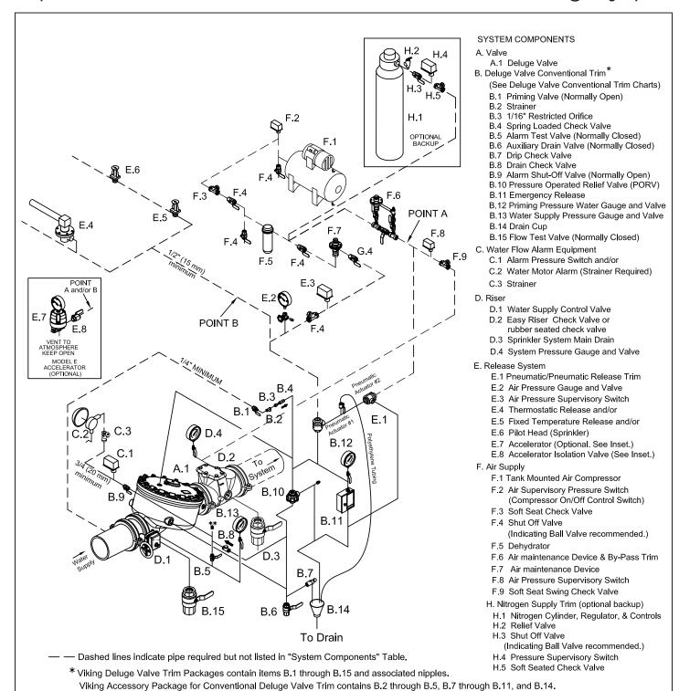
FIGURE 3: Straight Through Horizontal Valve with Tank-Mounted Compressor (6" Valve Shown)
