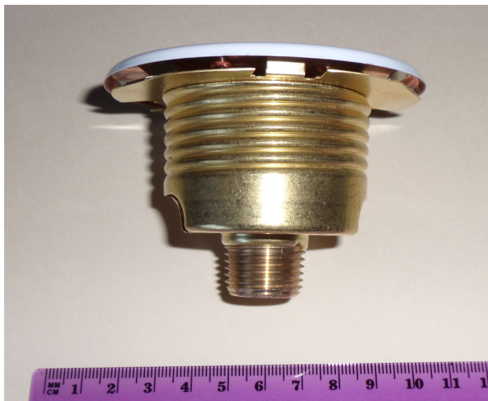
FIGURE 1. The VK462 with UNS-S43000 that underwent testing for translational attraction.
