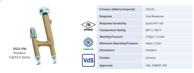
The DS21-FM preaction sprinkler unit consists of a housing with two separate sprinkler heads. Before water is released, both sprinkler heads in the unit must be triggered.
