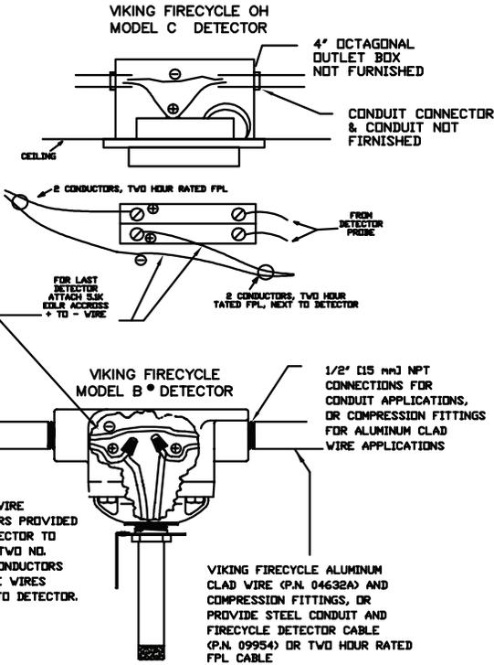
CERAMIC WIRE CONNECTORS PROVIDED WITH DETECTOR TO CONNECT TWO NO. 16 AWG CONDUCTORS TO SINGLE WIRES LEADING TO DETECTOR.
