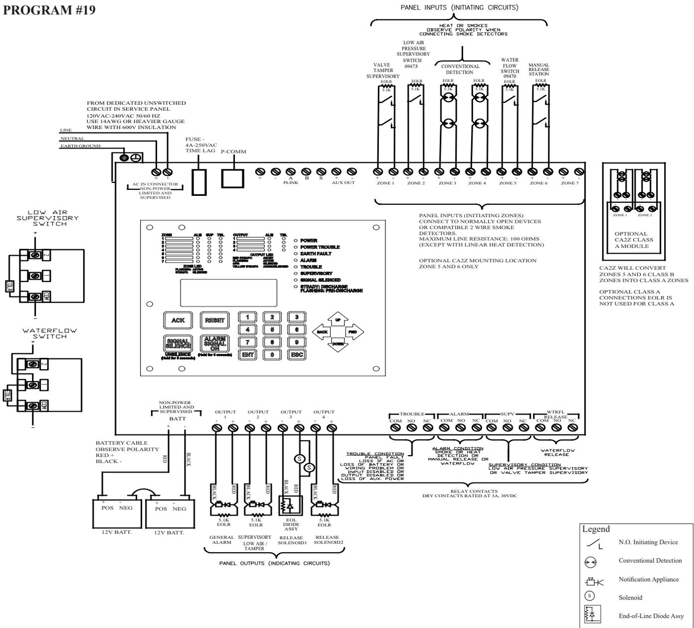
1. Run field wiring and ensure connections are proper by metering wires. Resistance reading should be 5.1K ohms with end-of-line resistor (EOLR) at last device. The end-of-line resistor are supplied with the panel. Install EOLR on all unused circuits.
