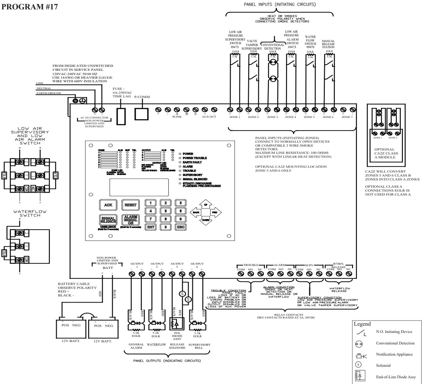
1. Run field wiring and ensure connections are proper by metering wires. Resistance reading should be 5.1K ohms with end-offline resistor (EOLR) at last device. The end-of-line resistor are supplied with the panel Install EOLR on all unused circuits.
