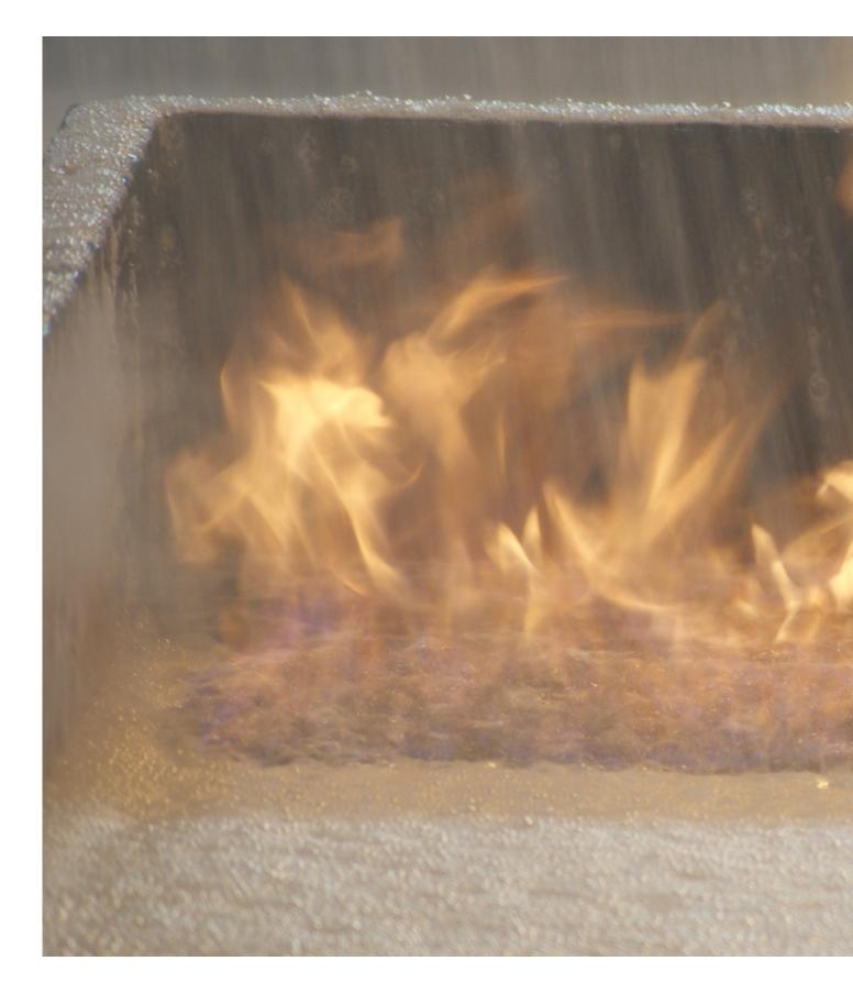
Non-aspirated foam sprinkler test according to Factory Mutual (FM) 5130 - Standard for Foam Extinguishing Systems.
