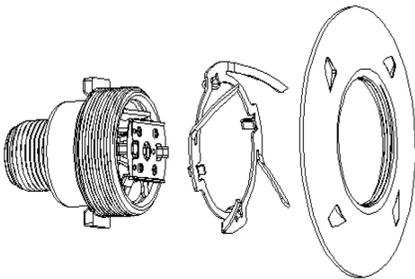
Figure 1- Institutional sprinkler with locking escutcheon ring.
