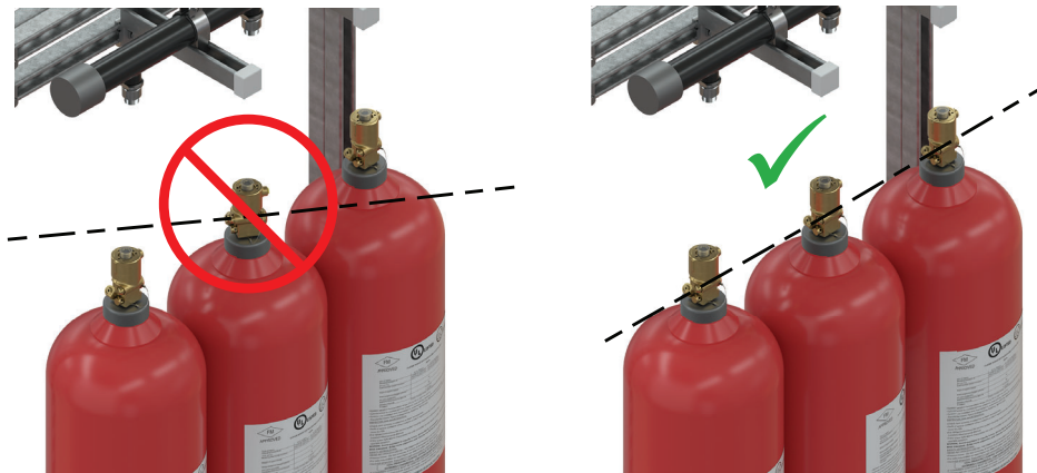
Figure 6.6: Align valve with manifold
