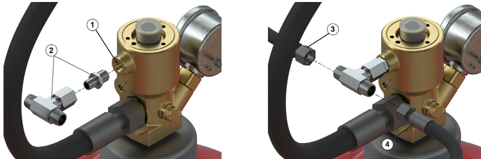
Figure 6.41: Install the pilot hoses between the cylinders
