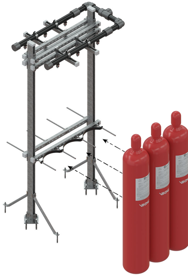
Figure 6.3: Position extinguishing agent cylinders
