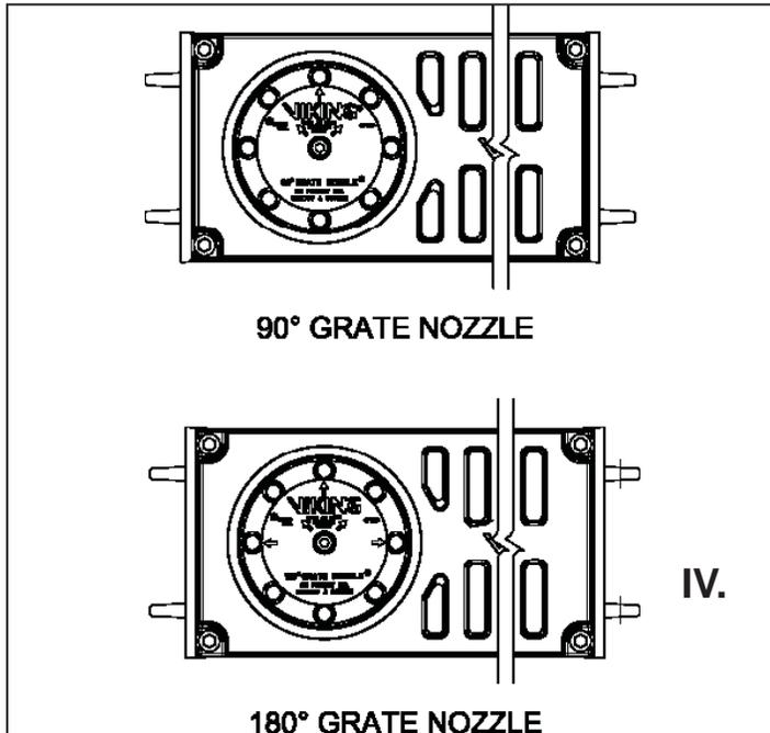
**Figure 24: 90° and 180° Grate Nozzles**
