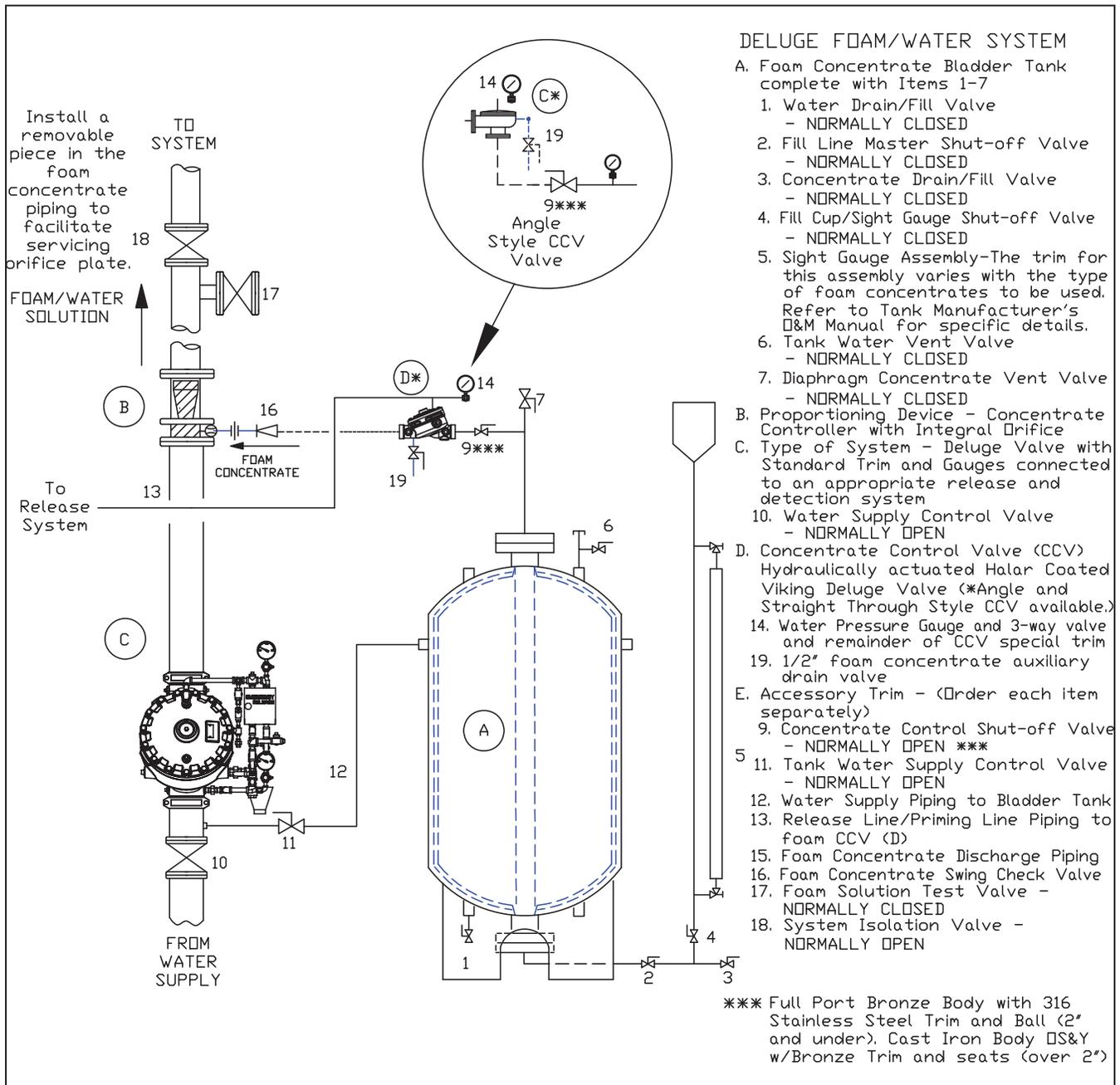
**Figure 10: Deluge Bladder Tank Foam-Water System**
