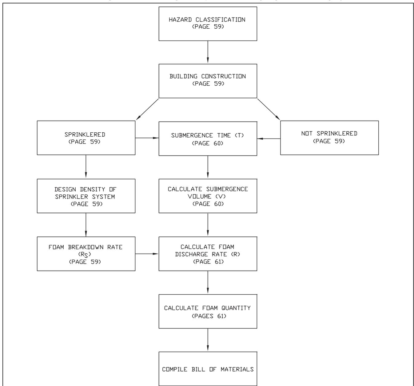
**Total Flooding High-Expansion Foam System Flow Chart**
