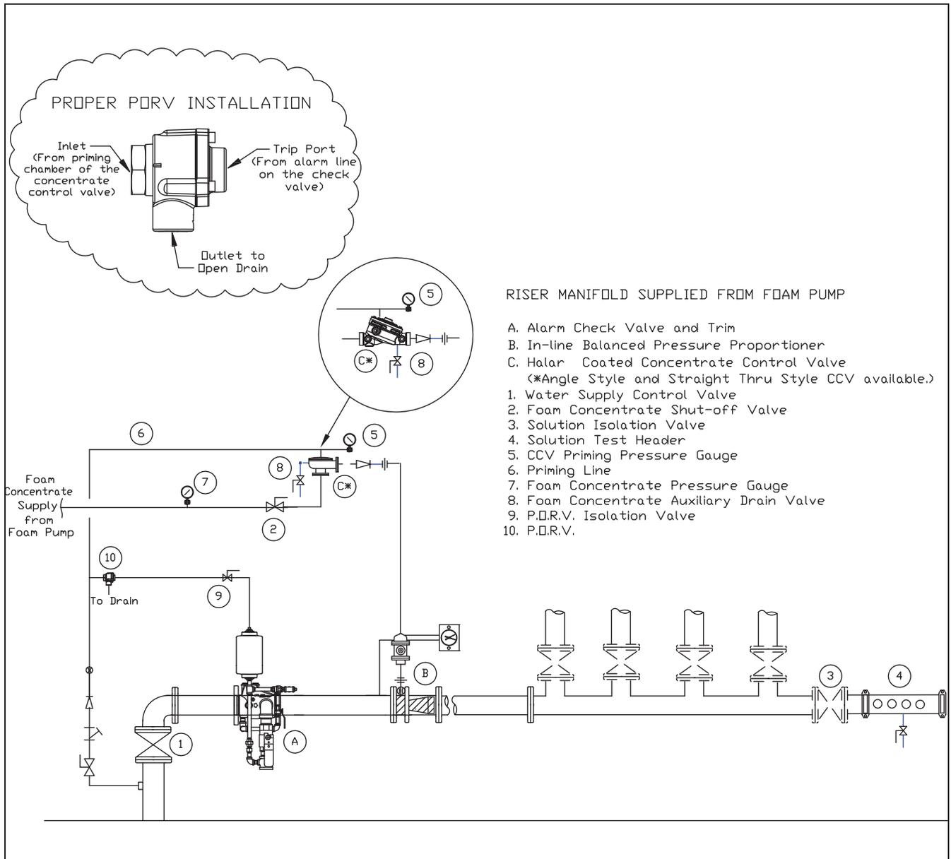
**Figure 4: Riser Manifold Supplied From Foam Pump**
