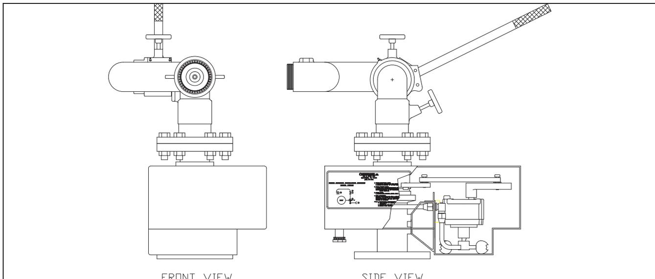
**Figure 20: Oscillating Monitor**
