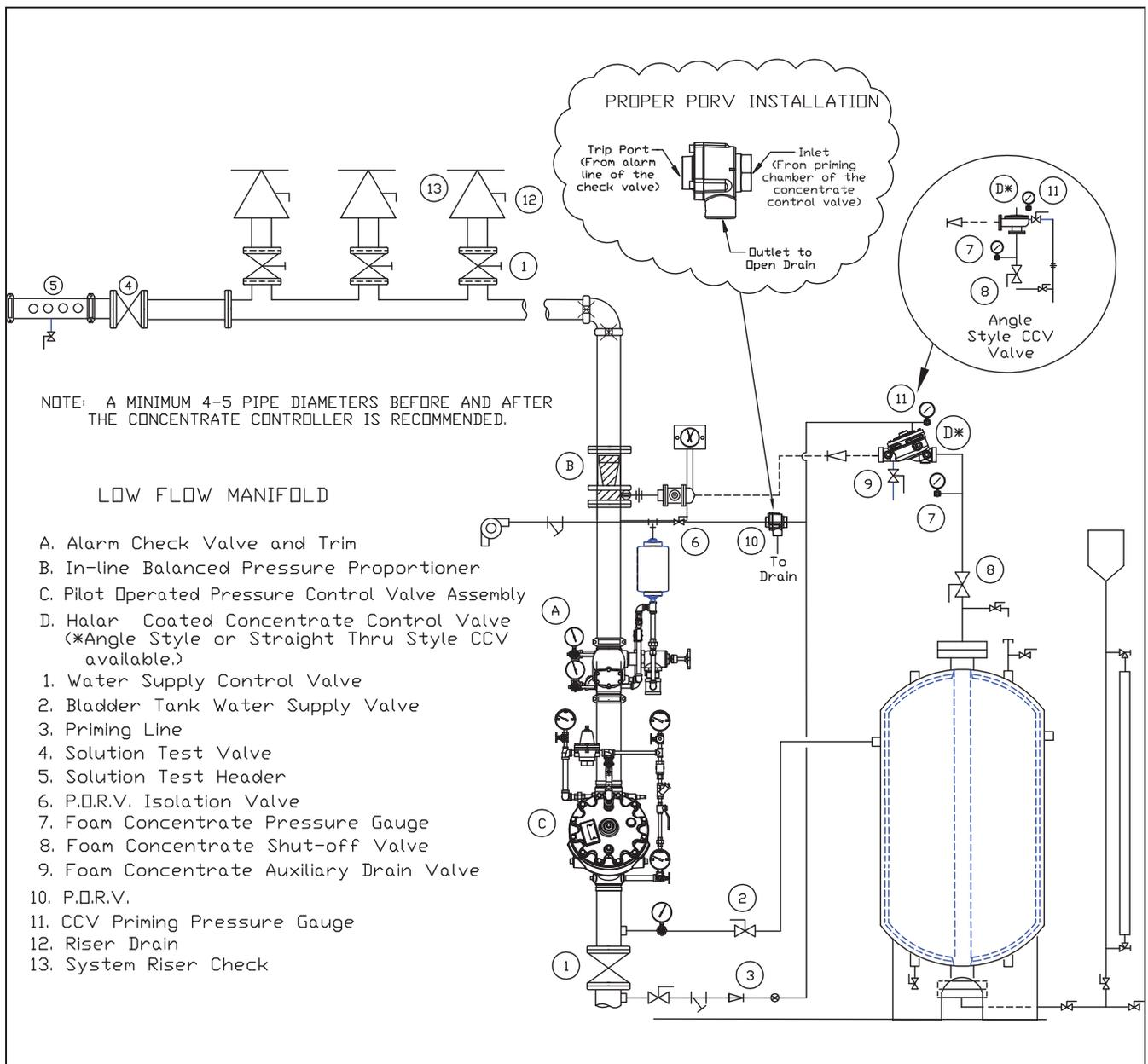
**Figure 6: Wet Pipe Low-Flow Manifold System**
