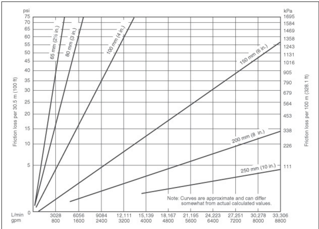
**Table 6: Expanded Foam Friction Losses vs Pipe Size (2-1/2" through 10")**
