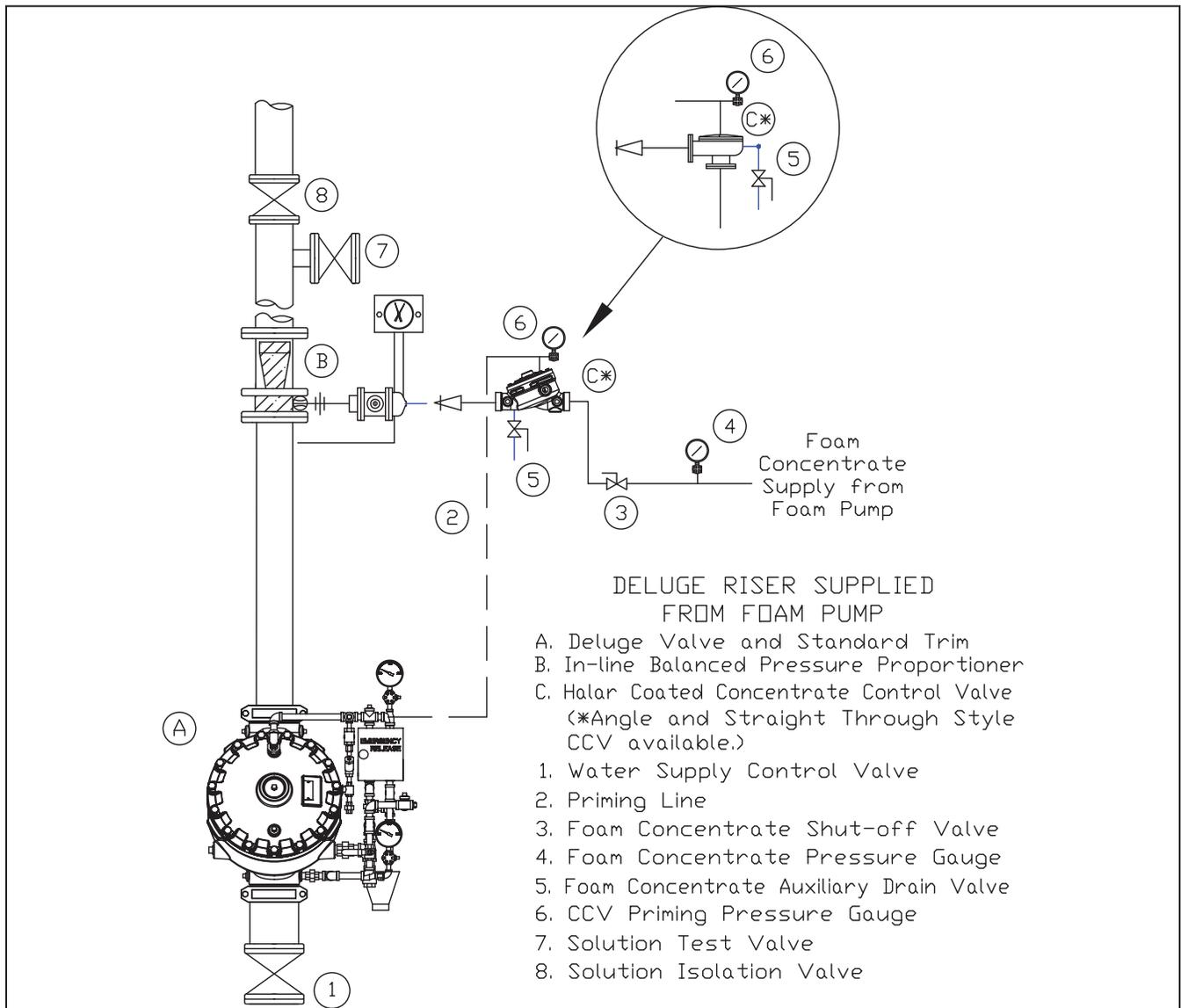
Figure 12: Deluge Riser Supplied From Foam Pump
