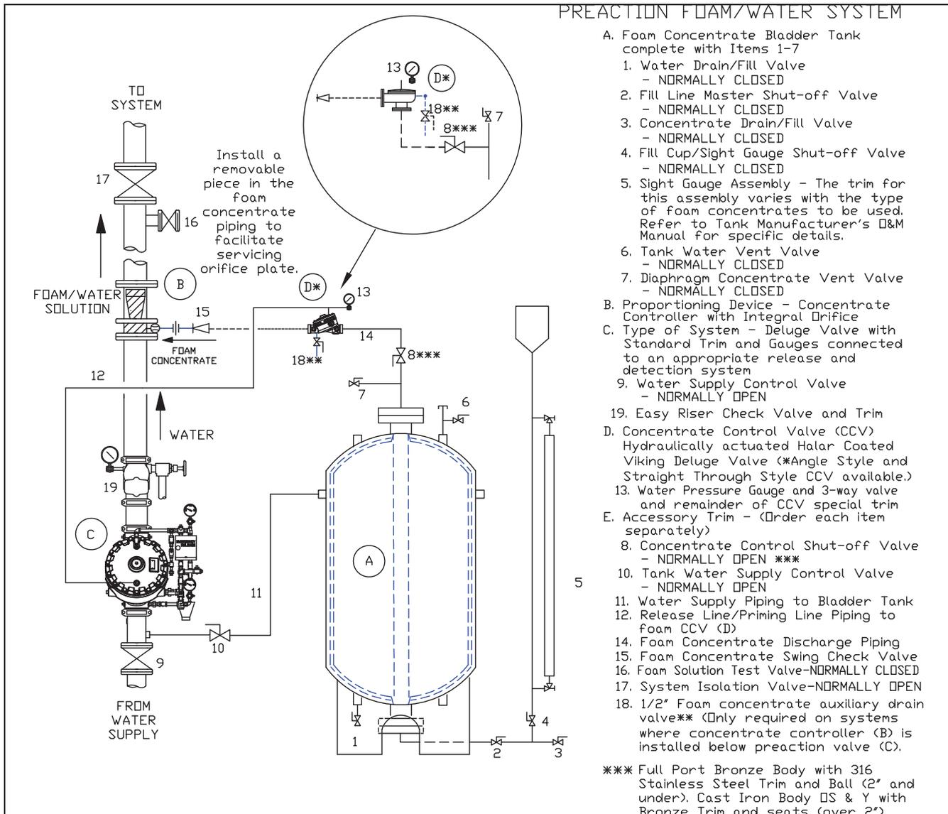
Figure 7: Preaction Bladder Tank Foam-Water System
