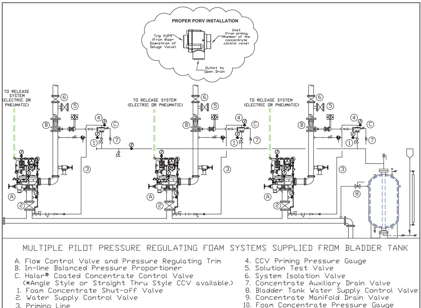
**Figure 14: Multiple Pilot Pressure Regulating Foam Systems Supplied From a Bladder Tank**
