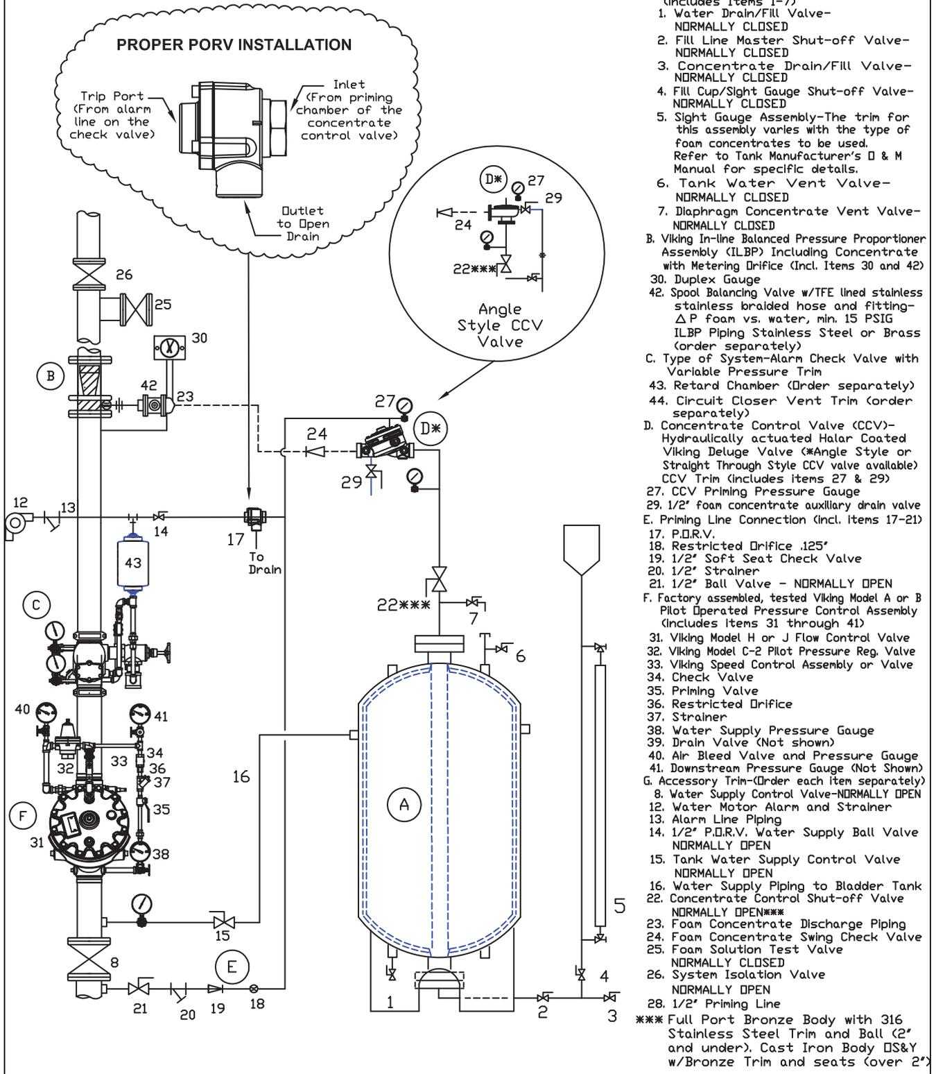
Figure 5: Wet Pipe Low-Flow Foam System Vertical Straight Through Pilot Operated Pressure Control Valve Assembly with Concentrate Control Valve
