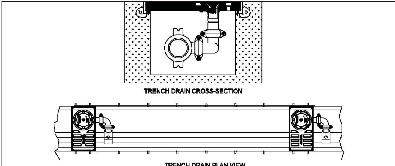
**Figure 26: Trench Drains**
