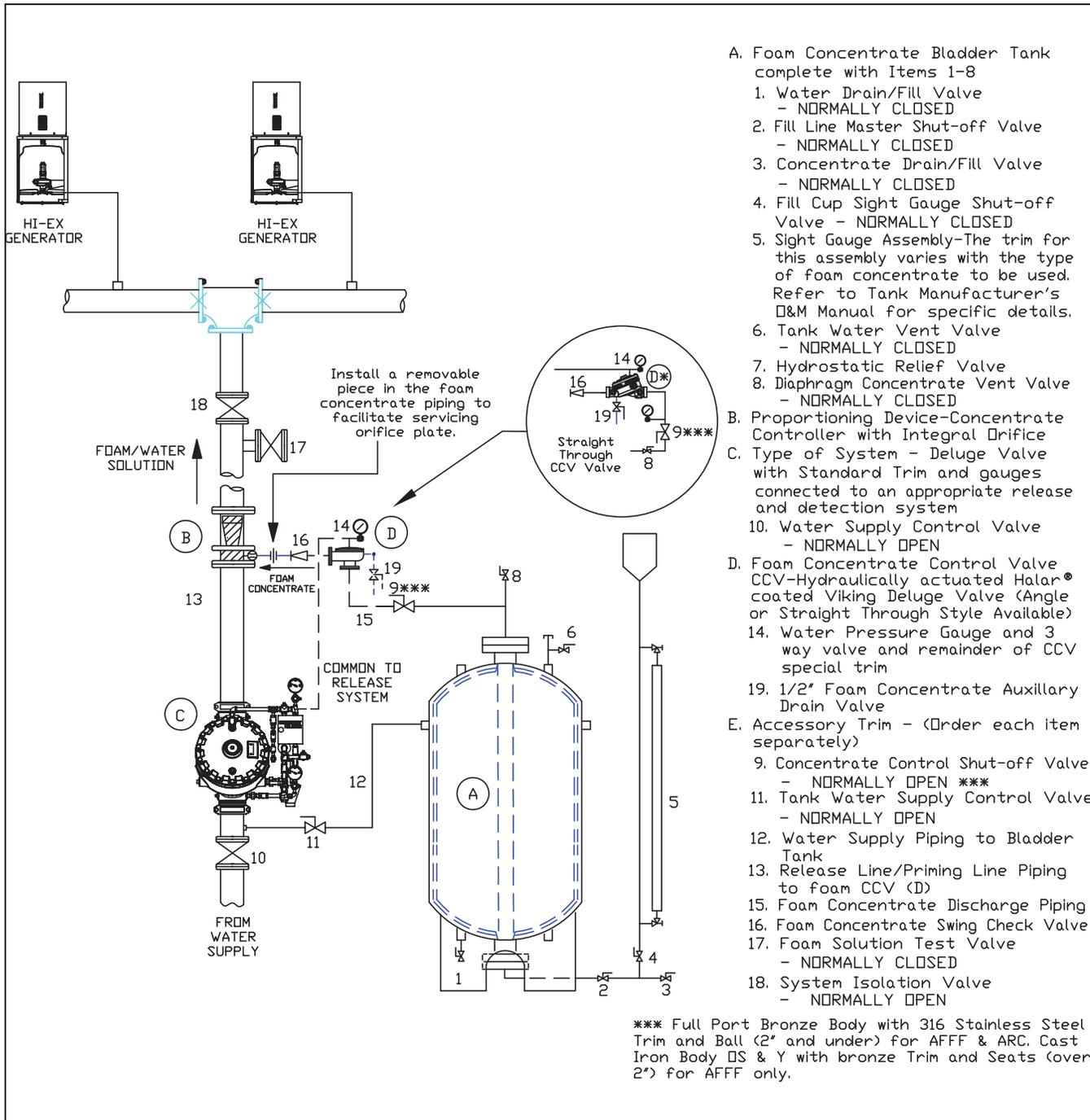
**Figure 16: High Expansion Foam System**
