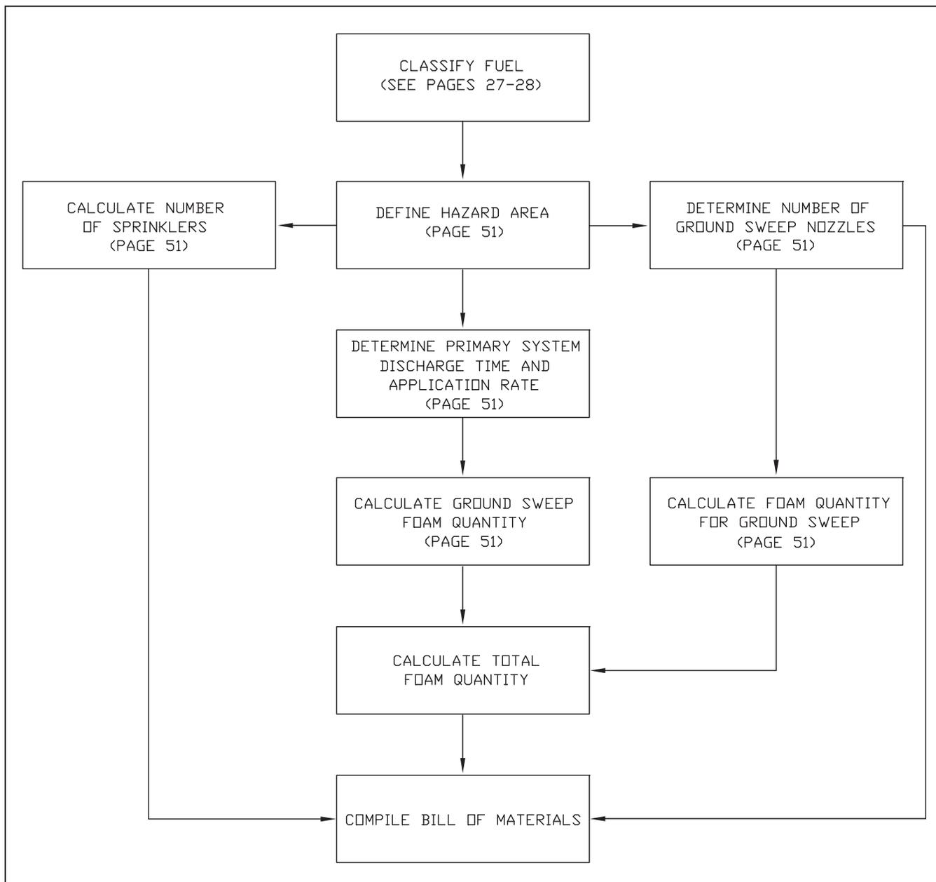
**Truck Loading Rack Protection Flow Chart**
