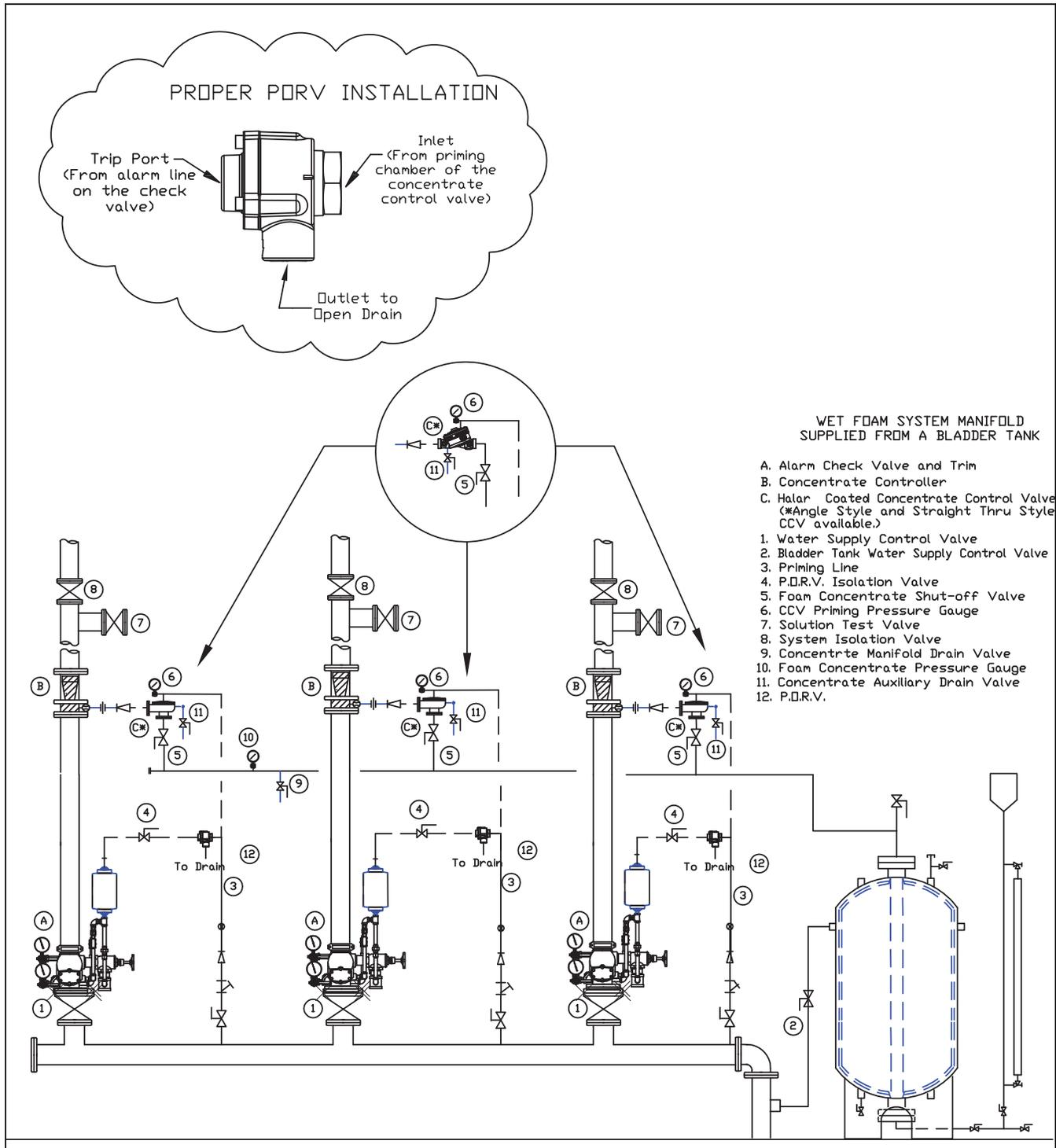
**Figure 2: Wet Foam System Manifold Supplied From a Bladder Tank**
