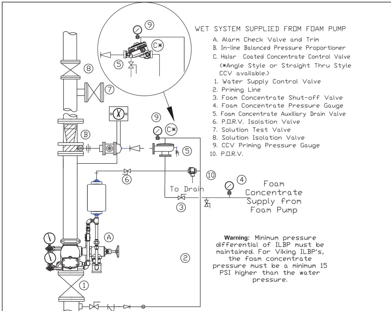
**Figure 3:** Wet System Supplied From Foam Pump
