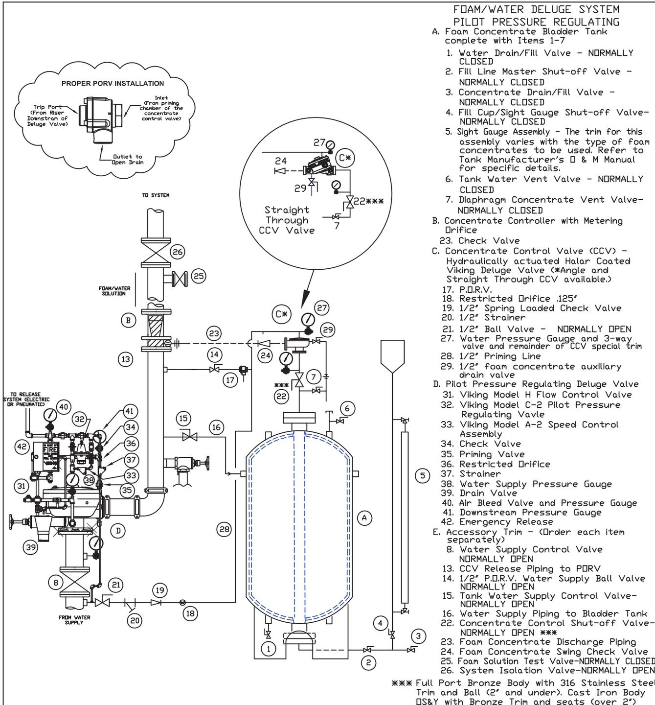
Figure 13: Pilot Pressure Regulating Foam-Water Deluge System
