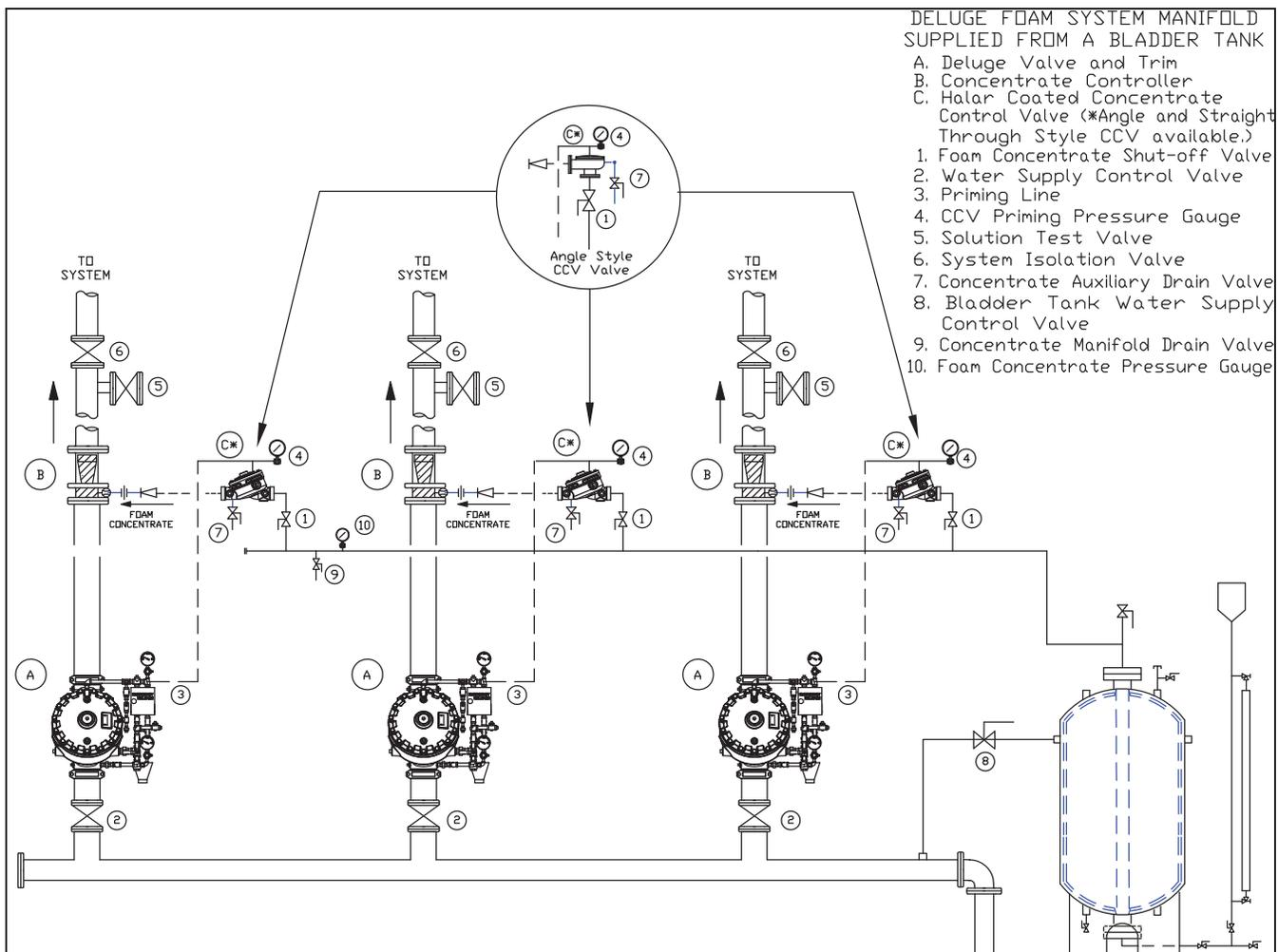
Figure 11: Deluge Foam System Manifold Supplied From a Bladder Tank
