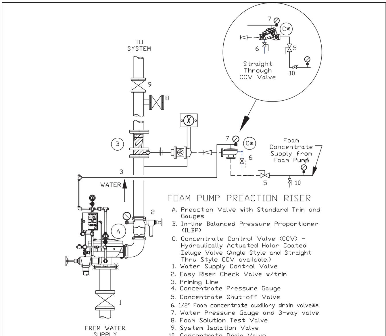
**Figure 8: Foam Pump Preaction Riser**
