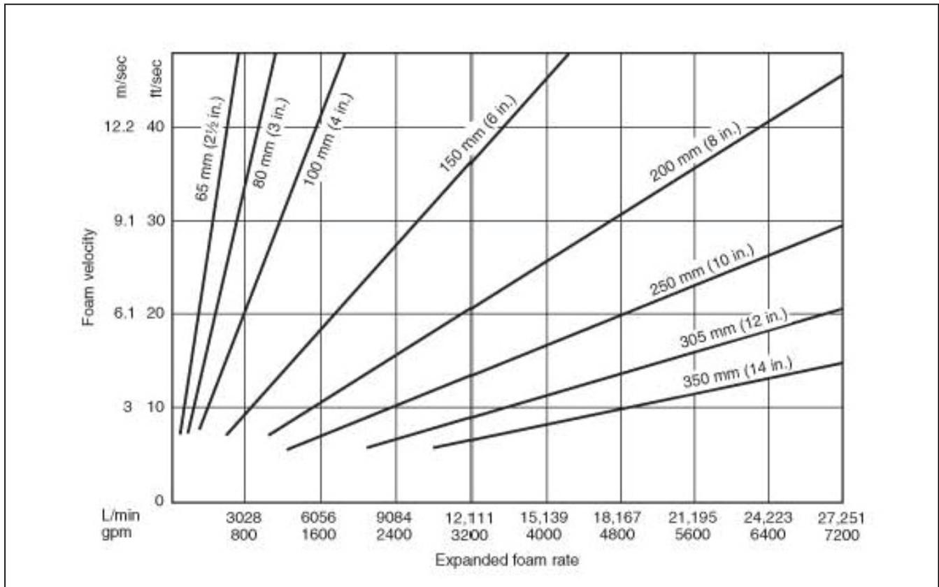
**Table 4: Foam Velocity vs. Pipe Size (2-1/2" through 14")**
