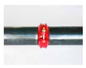
The nuts must be tightened evenly and by alternating sides, otherwise the gasket can become pinched and damaged, which can lead to immediate or subsequent leaks.
