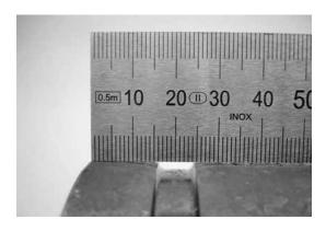
Measure the gasket seat length A and the groove width B using a ruler, a scale or a tape with linear scale to ensure the dimensions are within the tolerances specified in column 3 and column 4 of table 6.
