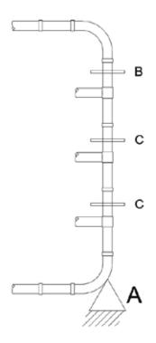
Install the riser with the predetermined gap method. Anchor the pipe at or near the base with a pressure thrust anchor "A" capable of sup- porting the full pressure thrust, weight of pipe and the fluid column. Anchor at "B" with an anchor capable of withstanding full pressure thrust at the top of the riser plus weight of pipe column. Place inter- mediate anchors "C" as shown, between anchors "A" and "B". Also place intermediate clamps at every other pipe length as a minimum.
