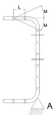
Install the riser with the pipe ends butted.
