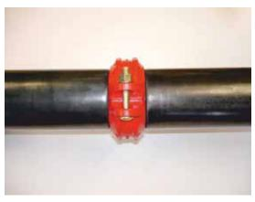
With the T&G style coupling no metal-to-metal contact of the bolt pads is required. You will normally see a 1.6 mm up to 3.2 mm (1/16" up to 1/8") gap between the bold pads when installed
