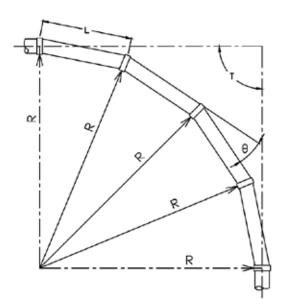
Utilizing the angular deflection at each coupling joint curves may be laid out using straight pipe lengths and Couplings.
