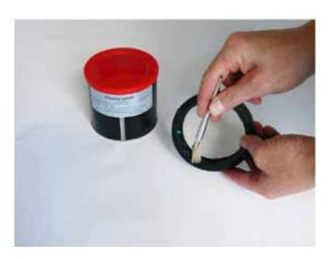
Cover the sealing lips and the outside of the gasket with a thin layer of lubricant.
