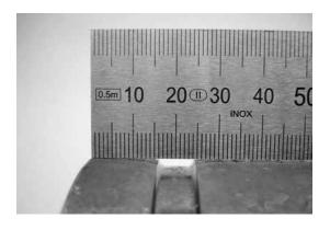
Measure the gasket seat length A and the groove width B using a ruler, a scale or a tape with linear scale to ensure the dimensions are within the tolerances specified in column 3 and column 4 of table 5.
