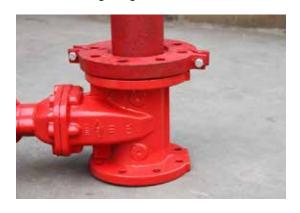
Align flange bolt holes with mating flange (or valve) bolt holes. Insert a standard flange bolt through bolt hole and hand tighten a nut. Insert another bolt opposite the first and hand tighten a nut. Continue this until all bolt holes are fitted. Tighten nuts evenly to specified bolt torque, so flange faces remain parallel. Assembly completed.
