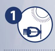
Protect all sprinklers from exposure to excessive heat - before, during, and after installation.
