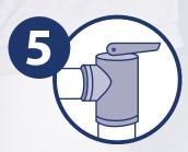
It is recommended to install a pressure relief valve whenever pressures may exceed the rating of any sprinkler system component.
