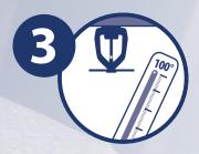
If exposure above 100° F is possible, use intermediate temperature-rated sprinklers per NFPA requirements.
