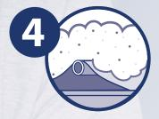
To separate excessive attic heat from sprinklers and piping, properly tent and fully insulate all pipe in unconditioned spaces.
