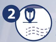
If exposure above 100° F is possible, install ordinary temperature-rated sprinklers only after protected space has been conditioned.
