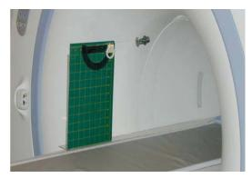
*Figure 4. Sprinkler with small deflection angle and, thus, low magnetic field interactions.*
