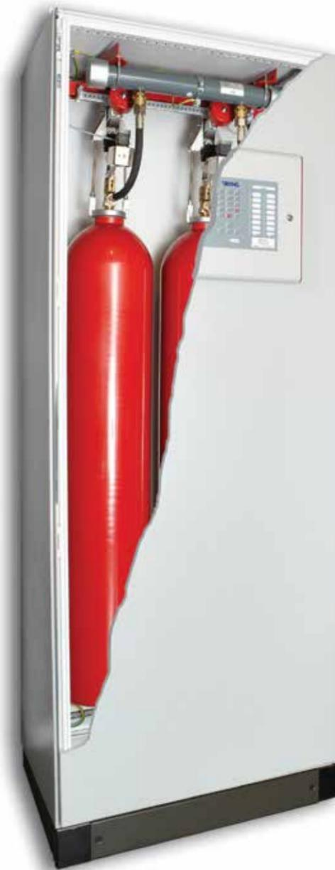
A fire detection control panel integrated in the front door is connected to the detectors, which react to heat or smoke, and activates the extinguishing unit in the event of a fire.
