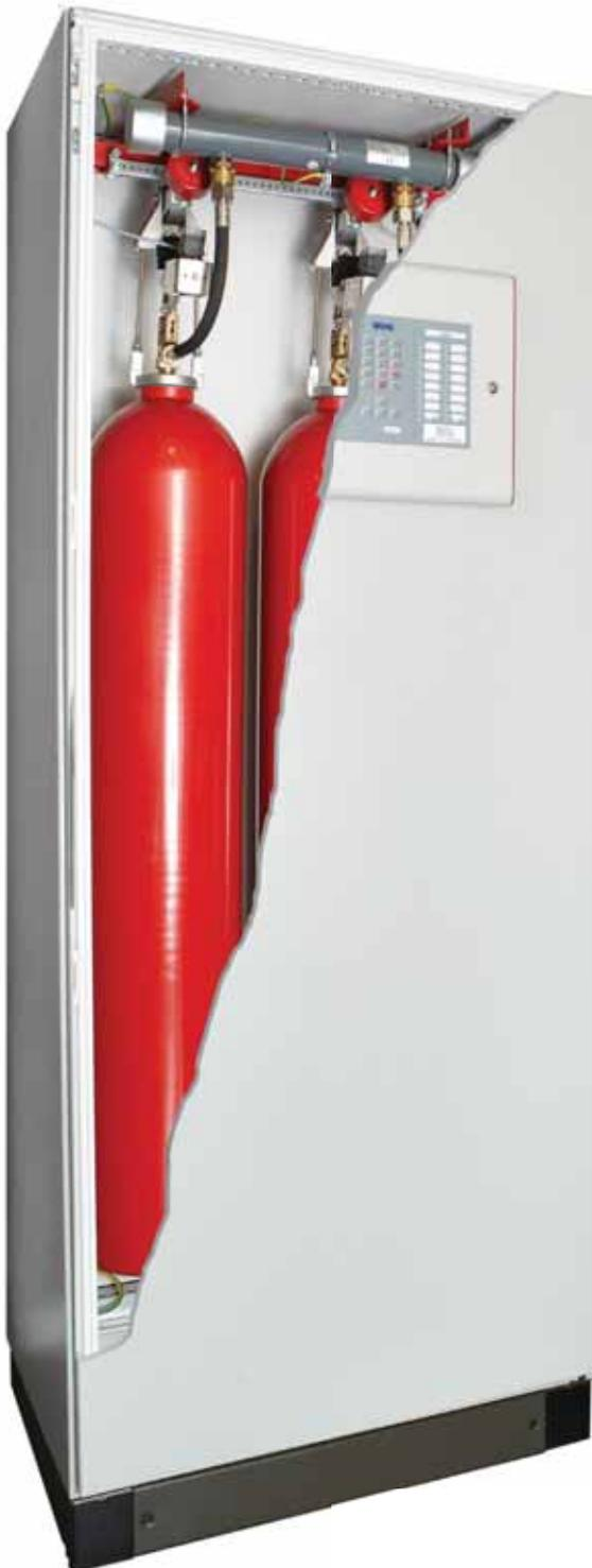
In compact assembling groups, all key components are combined in a cabinet to form a single unit that offers protection against dust and moisture or mechanical stress. The cabinet contains a rack with one or two extinguishing gas cylinders, an electronically monitored leakage indicator and an electromagnetic extinguishing agent activation device.
