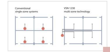
VSN 1230 fire extinguishing systems can be designed for use as a single-zone system to protect a single protected area or in the form of a multi-zone system to protect two or more areas.
