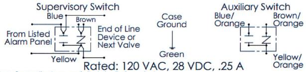
Wiring Notes: Connection to power limited circuitry is required.
