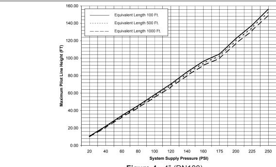
Figure 4 - 4" (DN100) Model F-1 Deluge Valves
