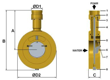
Figure 3.2.1: Components and Dimensions
