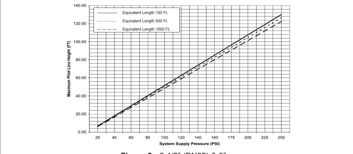
Figure 3 - 2-1/2" (DN65) & 3" (DN80) Model F-1 Deluge Valves
