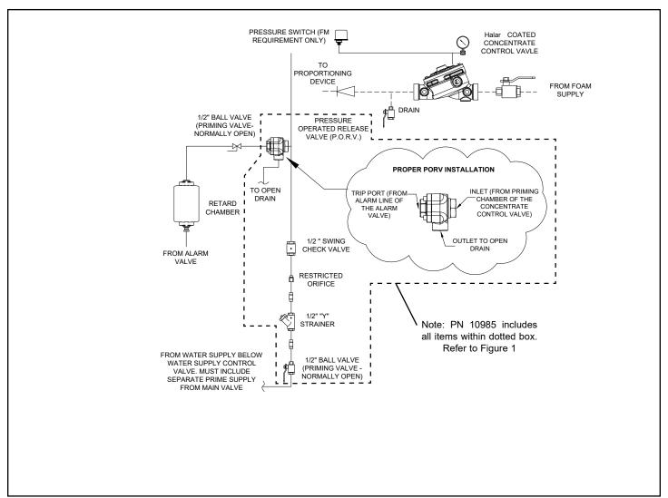
Figure 3 - Wet Pipe Foam Systems
