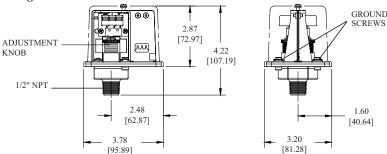
NOTE: To prevent leakage, apply Teflon tape sealant to male threads only.
