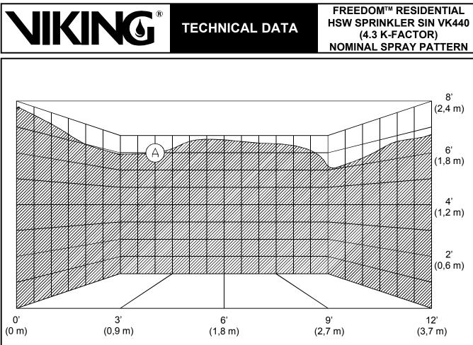
Typical profile of one half of the 12' x 12' (3,7 m x 3,7 m) spray pattern produced by a Viking Freedom<sup>TM</sup>  $\frac{1}{2}$ " (15 mm) Residential Horizontal Sidewall Sprinkler SIN VK440 installed with the deflector located 4" below the ceiling. Nominal U.S. K-Factor = 4.3 (6,2 metric).
