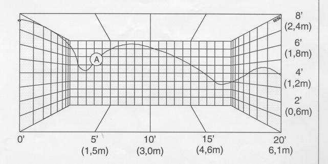
Typical profile of one half of the 16' X 20' spray pattern produced by a Viking 1/2" Extended Coverage Horizontal Sidewall Sprinkler.
