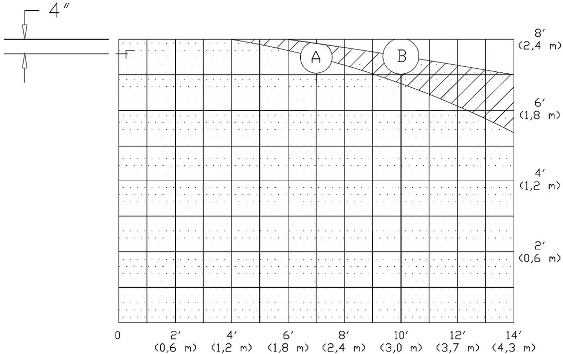
Typical side view of one half of the spray pattern produced by a Model Institutional Sidewall Sprinkler
