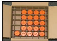
CORRECT (Protective caps in place)
