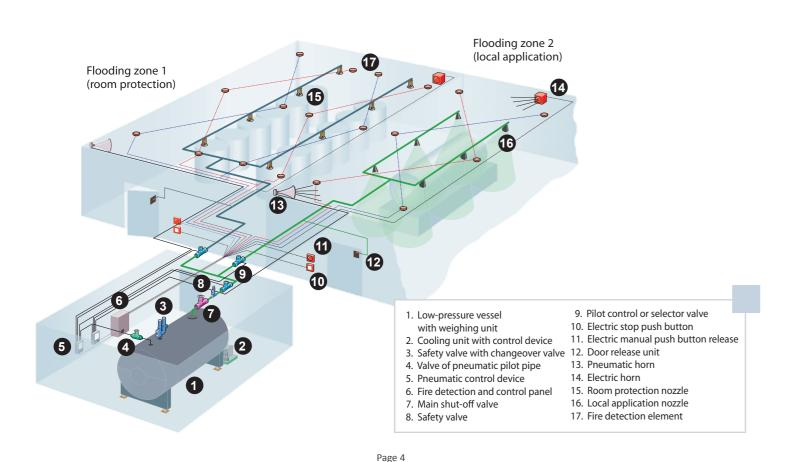
In pre-fabricated compact modules, all function-relevant components are combined with various functions in a single unit and accommodated in a protective cabinet, where they are protected from dust, moisture and mechanical damage. A compact module consists of a frame with freely suspended extinguishing gas cylinders, which are connected via pressure-proof hoses with the manifold, including weighing units with electronically monitored leakage indicators and an electromagnetic gas release.
