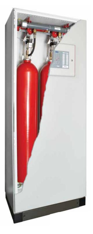
In compact assembling groups, all key components are combined in a cabinet to form a single unit that offers protection against dust and moisture or mechanical stress. The cabinet contains a rack with one or two extinguishing gas cylinders, an electronically monitored leakage indicator and an electromagnetic extinguishing agent activation device.
