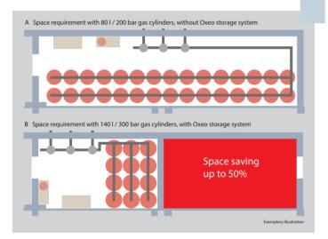
The possibility to arrange the gas cylinders in multiple rows and to adapt the cylinder setup to the premises creates additional flexibility for the inert gas storage. As a result, Oxeo extinguishing systems require up to 50% less space for the extinguishing gas supply than inert gas systems with 80 l / 200 bar gas cylinders and a conventional supply system.
